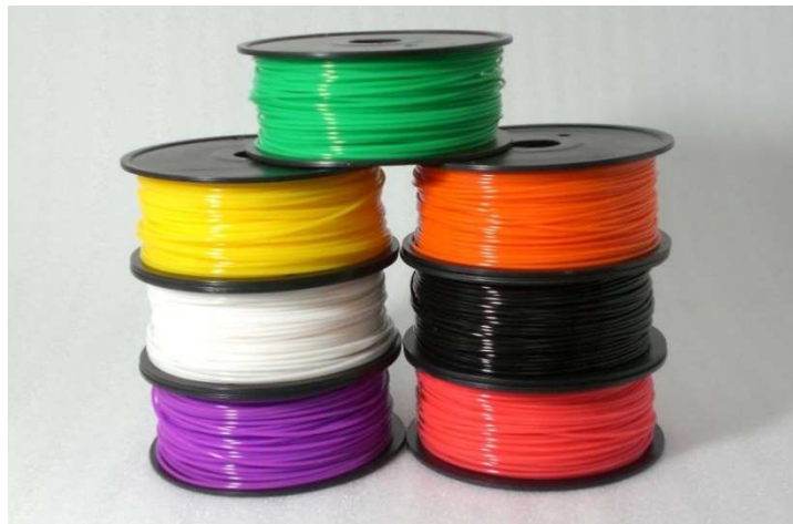
Figure 9. Rolls of plastic filaments is the main material used on 3D Printers
